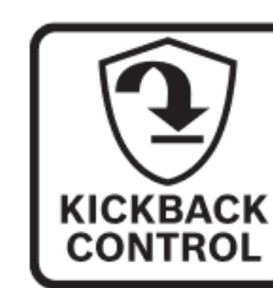
If there is a sudden kickback in the power tool, e.g. jamming in a separating cut, the power supply to the motor will be interrupted electronically.
