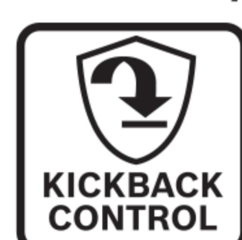
In case of a sudden drop in speed, e.g., caused by a jammed disc while cutting, the power supply to the motor is electronically interrupted.
