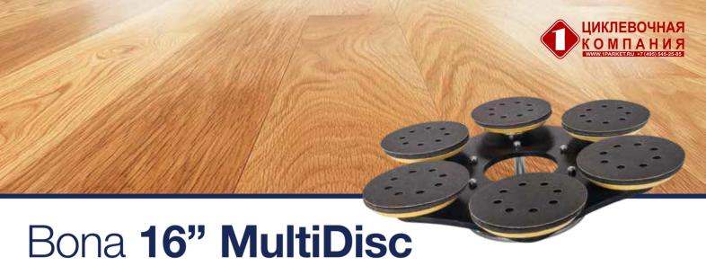
The Bona 16" MultiDisc is an innovative 6 disc drive plate that creates the perfect surface for a Bona Finish System. The six-5" discs spin independently of each other, eliminating swirls and scratch marks, leaving the floor smooth and flat. The Bona MultiDisc is perfect for patterned and dark stained floors and removing chatter marks. Provides the same performance around edges and detail areas to ensure no picture framing occurs. Compatible with most buffers.
