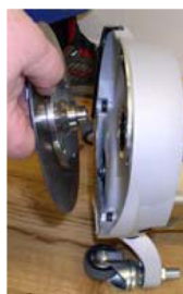
Remount the Velcro disc, pulley screw and the nut for the Velcro disc.
