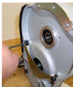
Replace the four screws. N.B. Do not tighten the screws!
