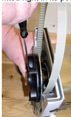
Tighten the screw and washer as well as the stop screw
