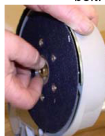
Remount the Velcro disc, pulley screw and the nut for the Velcro disc.
