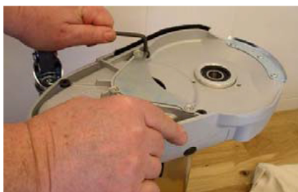
Tighten the four screws while holding the sanding arm in its position.
