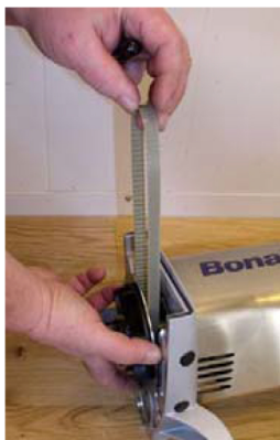
Mount a new belt together with the ventilator and cover plate.
