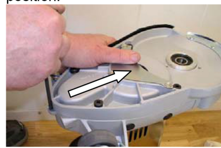
Place a screwdriver in the hole and press forward to tighten the belt.
