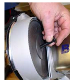
Remount the Velcro disc, pulley screw and the nut for the Velcro disc.
